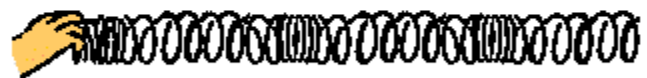
When the first coil of the slinky is repeatedly vibrated back and forth, a disturbance is created which travels through the slinky from one end to the other.
