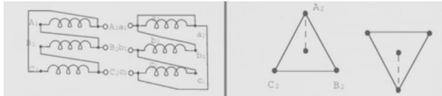
Fig 4.11 Dd6 connection and phasor diagram
