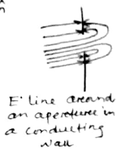
Electric field lines around a aperture. Electric polarization current normal to conducting wall
